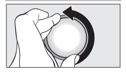
Turn the light cover counterclockwise and pull out. Never touch a halogen bulb with bare fingers.
